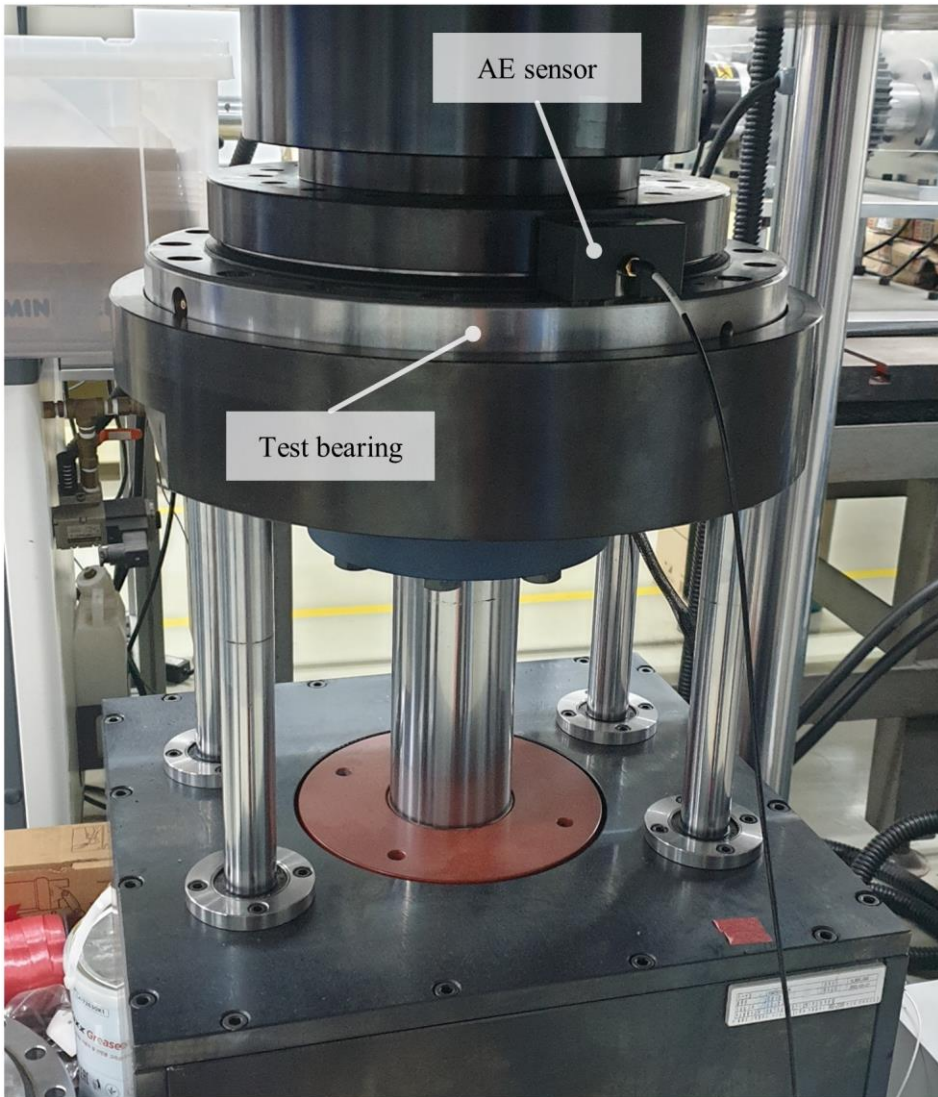
Figure 3-3 Slewing bearing test rig: (a) overall configuration of the test rig, and (b) data gathering through the AE sensor.
