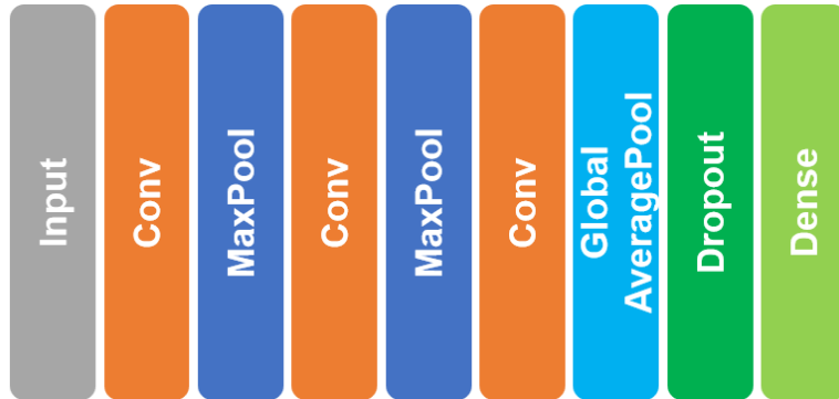
Figure 4-4 Neural architecture of 2D-CNN.
