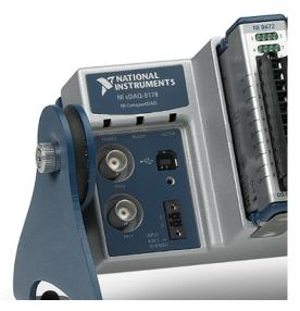
Figure 5. NI cDAQ-9178 Connections Showing BNC Triggers, Flexible Power Connector, and USB Port with Threaded Hole for Cable Strain Relief
