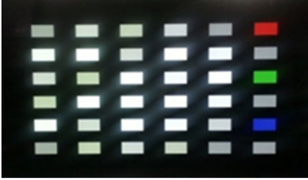
Fig. 2. Pattern of the ADT: the display size is 55 in; the number of pixels is 1920 \times 1080 ; and the number of pixels in an individual pattern is 160 \times 96 .
